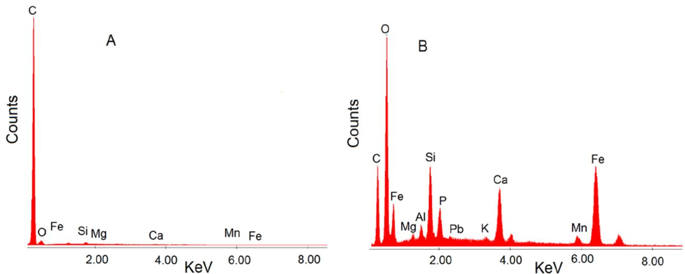
Figure 2: Elemental composition of **A.** Fresh plastic filter media indicating the presence of carbon as major element and **B.** Coated plastic filter media from Filter 2 indicating the presence of iron and manganese along with other elements through X-ray detector (Energy Dispersive Spectrometer).
