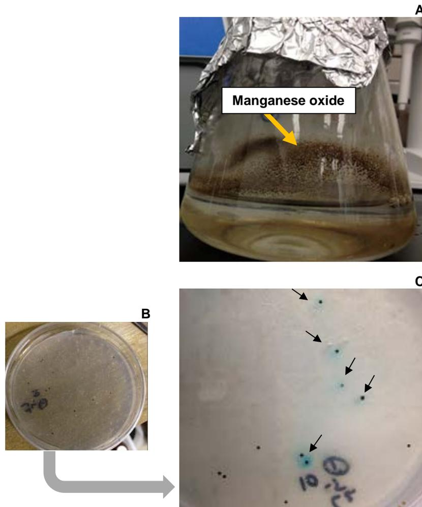
Figure 3: **A.** The culture-dependent microbial assessment of manganese-oxidizing bacteria in optimized nutrient media; the yellow arrow points to the brown layer formed on the walls of the flask, which was qualitatively confirmed to be composed of manganese oxides using the leucoberberlin blue test. **B.** The
