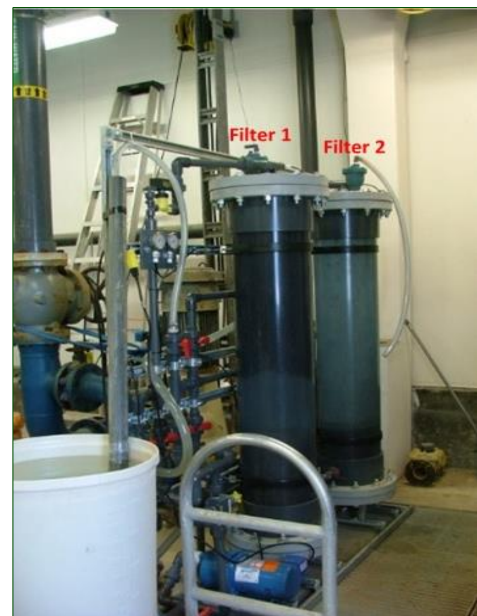
On-site pilot-scale biofiltration unit at the Langham Water Treatment Plant (Filter-1: Fe-biofilter; and, Filter-2: Mn-biofilter)
